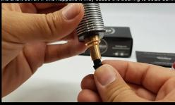
7) Once you have given the pinion ample time to dry on the shaft, put a small blob of Loctite on the grub screw and secure this in the pinion. Tighten the grub screw until firm, but do not over tighten. now leave the Loctite / adhesive to set for the correct amount of time according to the instructions for the product.
