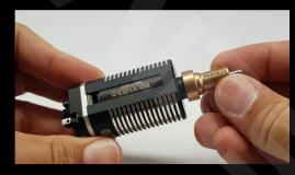
3) The second step is to remove the small pieces of heat shrink from the connector tabs at the back of the motor. These are not required to be removed prior to use. To do this use a small flathead screwdriver or another appropriate tool. Use care when doing so to prevent damage to the connector tabs on the motor. Once removed you can discard the heat shrink.
