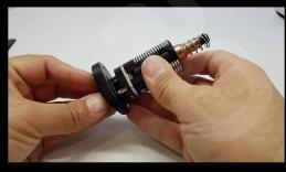
9) Checking the fitment in this way will ensure you have the correct engagement angle when your motor is fitted inside your gun. Perform any modification or filing that is required to the pistol grip prior to use in your AEG. Once you have completed this last step you are ready to fit the motor.
