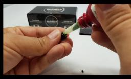
6) It is important when sliding the pinion onto the shaft that you should hold the motor with the shaft facing downwards. this prevents the Loctite you have used form getting into the bearing on the shaft cover. If this happens it may cause the bearing to seize during operation.
