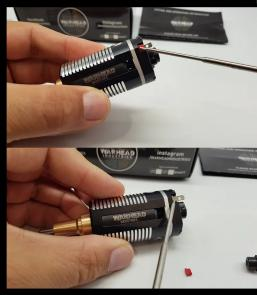
4) Once the shaft cover is in place you are ready to attach the pinion. Remove the grub screw in the pinion using a 1.27mm allen key / hex driver.
