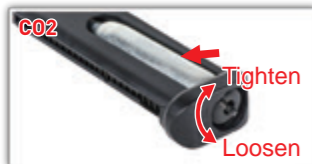
Use 6mm allen wrench to loosen the CO2 cartridge tray. Install the CO2 cartridge then tighten the tray.
