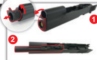
1. Flip the slide over and turn the barrel plug counter clockwise to remove it. 2. Remove the barrel.
