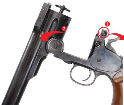
Push back the barrel latch and rotate the barrel downward. With the barrel pointed in a safe direction, continue to open the frame and barrel until the extractor completes its cycle and snaps back into the cylinder.
