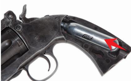
Load the CO<sub>2</sub> capsule into the CO<sub>2</sub> compartment.
