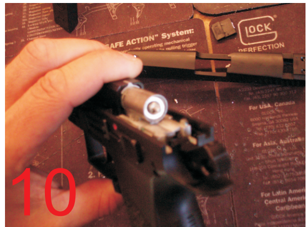
Valve-assembly seen from the back
